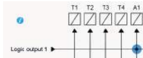
Figure 169 - An example of output matrix configuration for trip circuit supervision with two digital inputs
