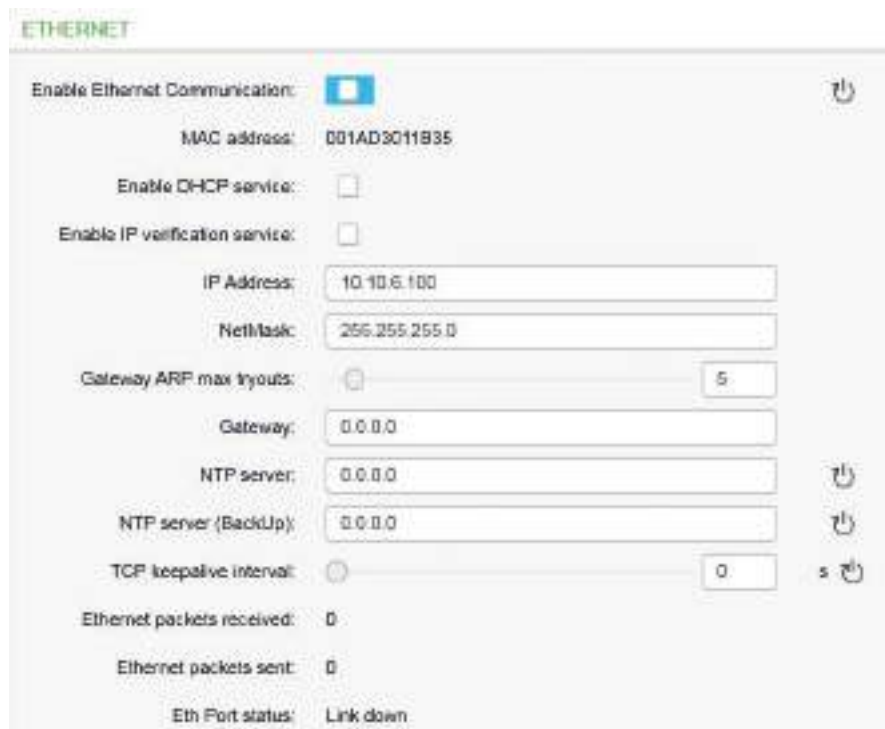
Figure 172 - Disabling the Ethernet port
