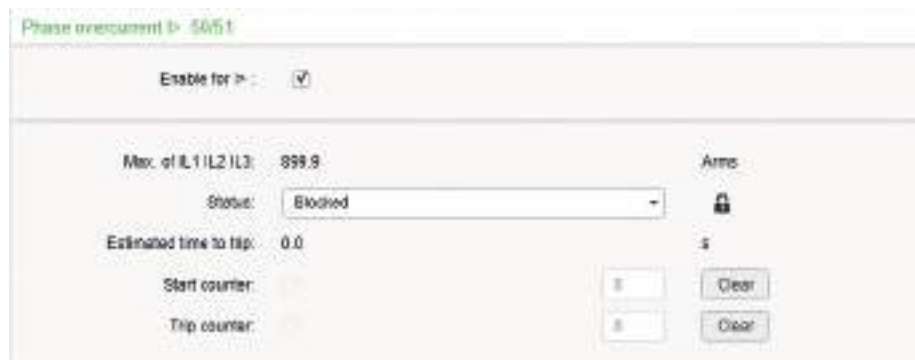
Figure 29 - Result for the I> stage when the DI is active and the stage exceeds its current start value
