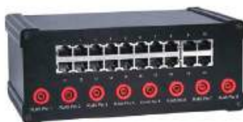
Figure 267 - LPIT test box
