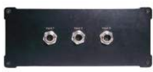
Figure 268 - The rear panel of LPIT test box
